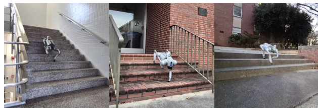
Figure 14: Stairs Climbing. LAPP-trained policies enable the Unitree Go2 robot to climb up and down stairs in a real-world deployment. The stairs are approximately 17 cm in height.
