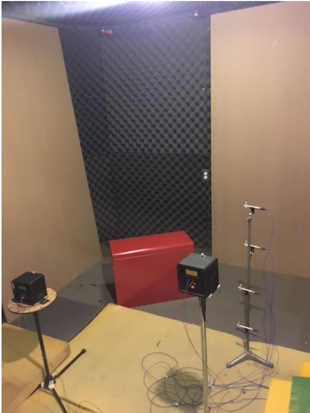
Fig. 1: Experimental setup. Pictured are two speakers (sources), two reflecting walls.
