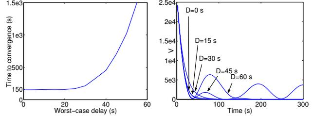
Fig. 7. Simulation results for a ten-agent wedge-shaped formation. Left: Time to convergence vs. the worst-case delay  $D$ . Right: Evolution of the Lyapunov function  $V$  for  $D$  equal to 0, 15, 30, 45 and 60s.
