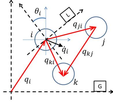
Fig. 2. Representation of the quantities used in the control law for agent  $i$ , expressed in an arbitrary global frame  $G$ . Three agents  $i$ ,  $j$  and  $k$  are depicted, and the local frame  $L$  of agent  $i$  is shown.
