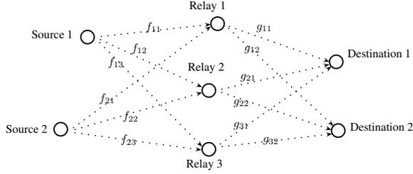
Fig. 1. Collaborative beamforming between 2 source-destination pairs via 3 relays. The signal transmitted from source 1 is intended for destination 1, while the signal transmitted from source 2 is intended for destination 2. Signals from sources 1 and 2 that reach destinations 2 and 1, respectively, are considered interference. Shown are also the channel gains  $f_{ij}$  between sources and relays and  $g_{ij}$  between relays and destinations.
