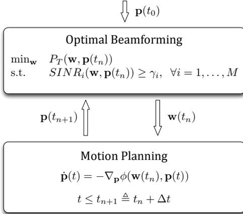
Fig. 3. Joint beamforming and mobility control.
